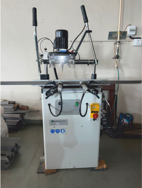
Copy Router To create Lock Sections
